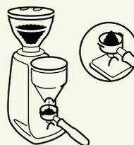
5. Flush water from the group head (the part of the machine where the portafilter locks in) for a few seconds before reinserting the portafilter.
