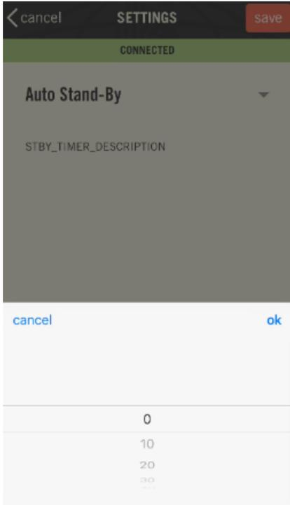
In the auto stand-by section, you can select the amount of time after which the machine will go in stand-by mode.
