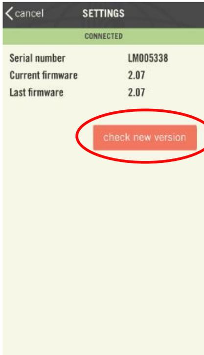
From the information section, it is possible to see the serial number, current firmware and it is also possible to verify if any newer firmware version is available.
