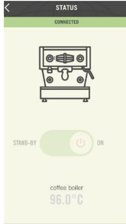
In the status display, it is possible to select the stand-by mode and to view the boiler temperature.
